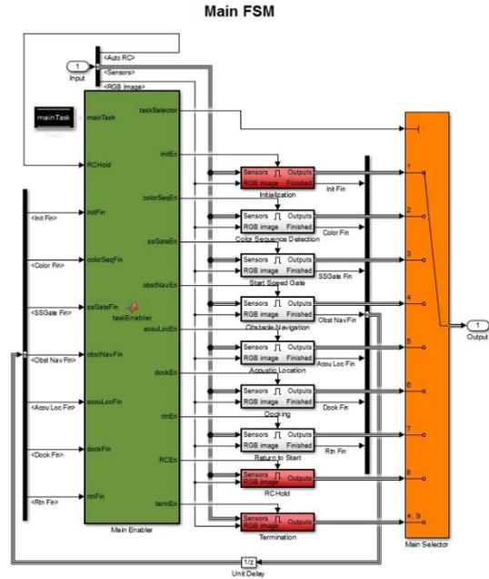
Figure 6: Structure of the Finite State Machine
