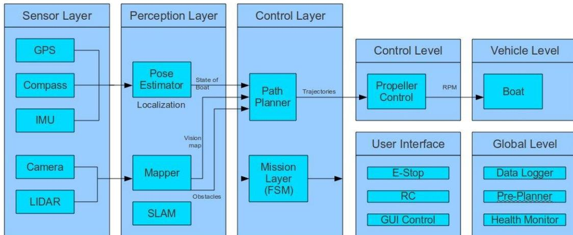
Figure 3: Flow Chart of SeaCat Logic
