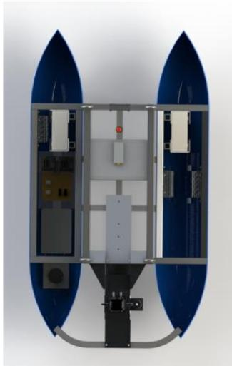
Figure 2: Top View of SeaCat with Location of Internal Components
