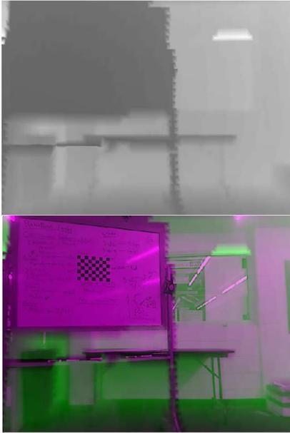
Figure 5: (Upper) Depth Map from LIDAR, (Lower) LIDAR and Video Fused Image
