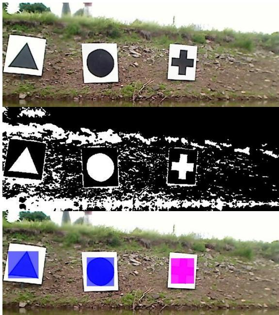
Figure 7: (Top) Original Video Frame, (Middle) Brightness Based Binary Mask, (Bottom) Template Detection with Cruciform Recognition
