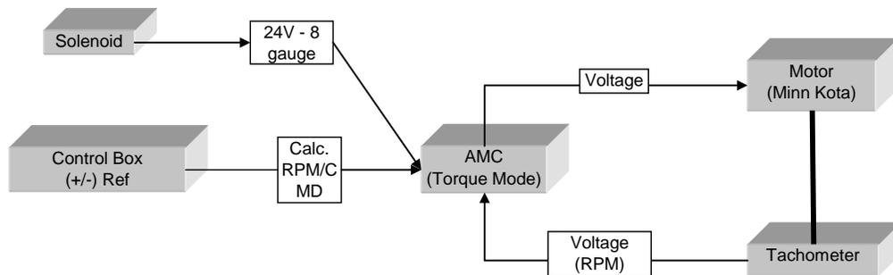
**Figure 6: Propulsion Block Diagram**
