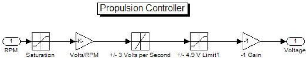
**Figure 5: Propulsion Control Diagram**
