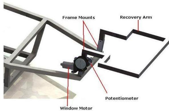
**Figure 14: Recovery System Open**
