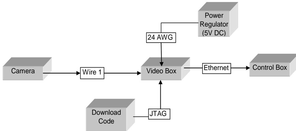
**Figure 25: Video Block Diagram**
