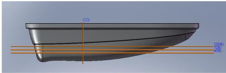
**Figure 3: Center of Gravity and Waterline for Different Weight**
