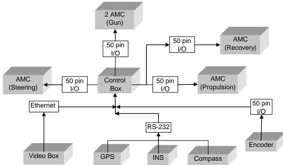
**Figure 18: External Control Box Block Diagram**
