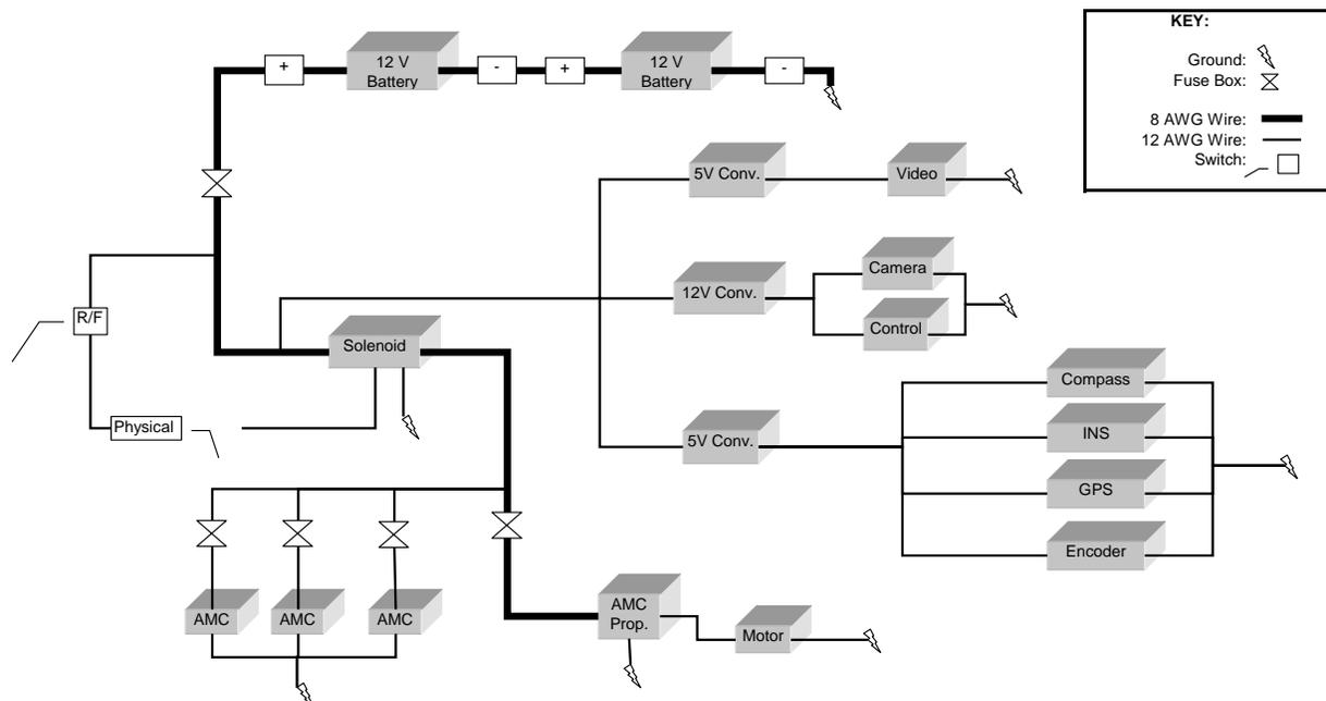
**Figure 16: Electrical System Block Diagram**
