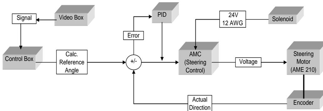
**Figure 9: Steering Block Flow Diagram**
