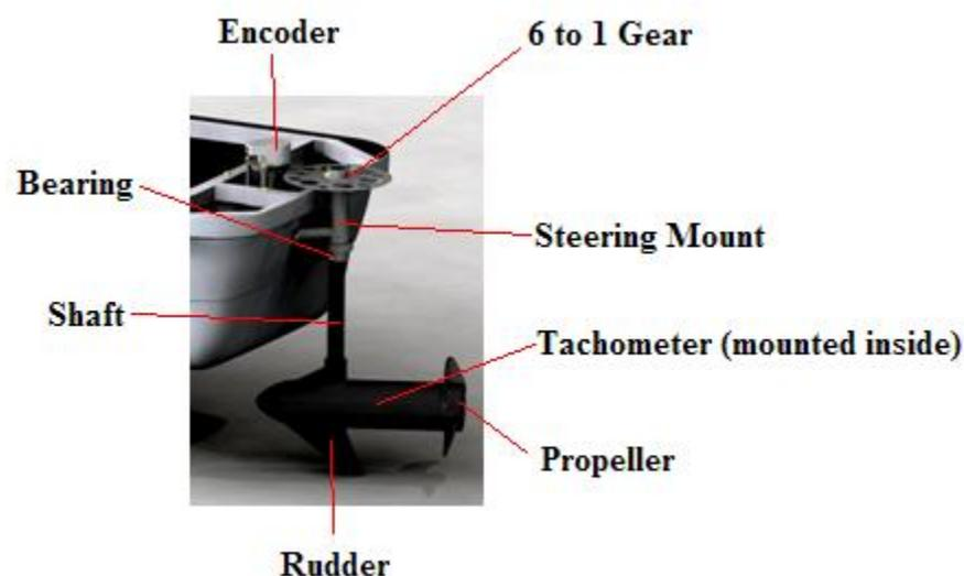
**Figure 7: Motor Mount and Steering System**
