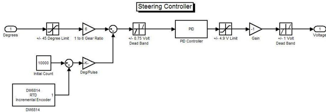
**Figure 8: Steering Control Diagram**
