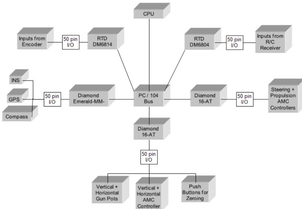
**Figure 19: Internal Control Box Block Diagram**
