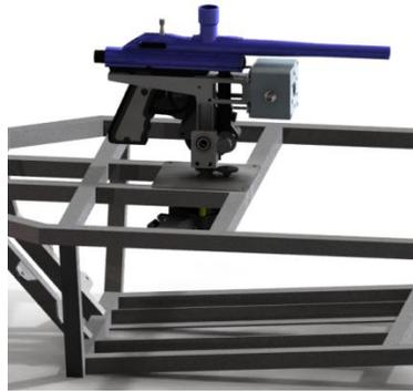
**Figure 12: Weapon System mounted in frame**
