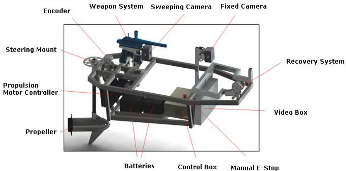
**Figure 1: Rendering of complete assembly**
