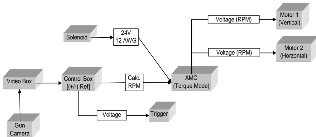
**Figure 11: Defense System Block Diagram**
