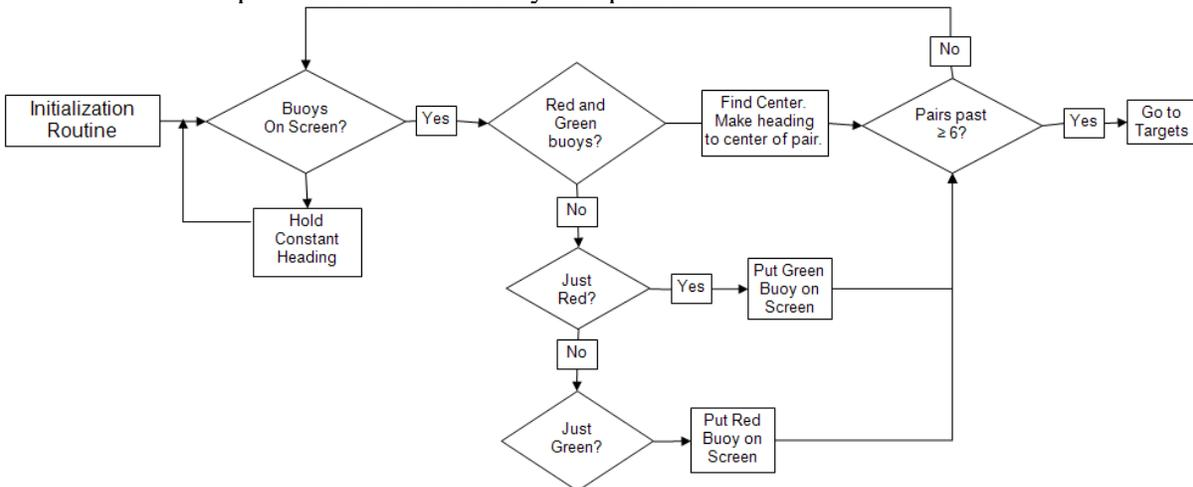
**Figure 21: Buoy Navigation Routine**
