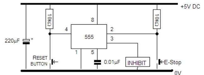
Figure 4: E-stop Circuit
