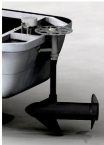
Figure 2: Motor mount and steering system
