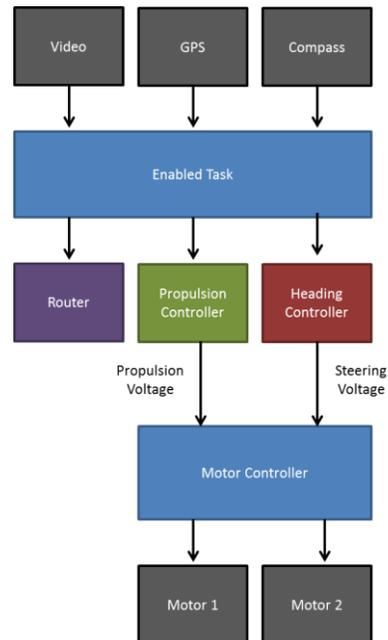
Figure 4: Diagram of SeaCat Logic
