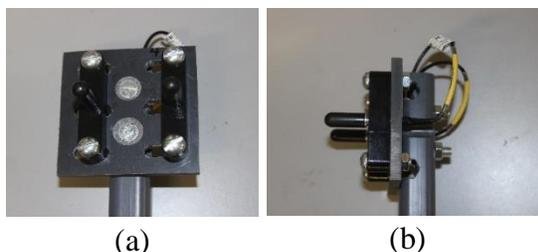
**Figure 6:** Hydrophone assembly, (a) front view and (b) side view.
