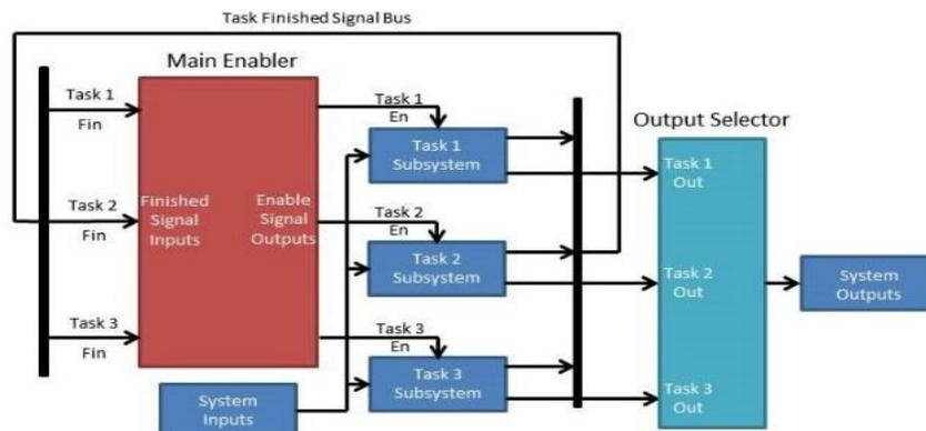
**Figure 7:** Structure of the Finite State Machine.
