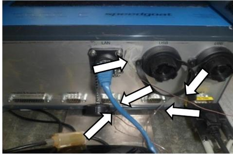
**Figure 5:** Thermocouples attached to the Speedgoat.
