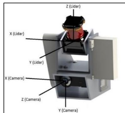
**Figure 2:** Vision System Assembly.
