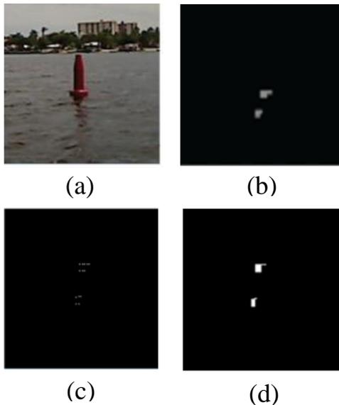
**Figure 3:** Example images showing video fusion. (a) The original RGB image, (b) raw LIDAR data, (c) LIDAR data plotted with respect to pixel indices, (d) joined LIDAR data creating a region of interest in the pixel frame.
