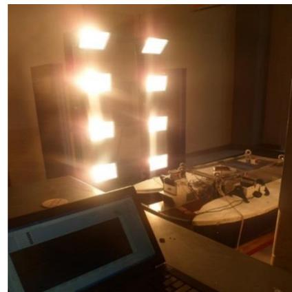
**Figure 4:** Experimental set up, solar emulator on with heat sink installed.
